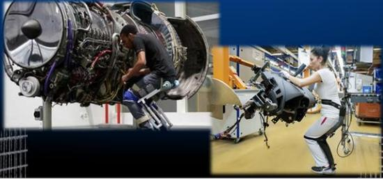
Noonee—a startup based in Switzerland—has created the Chairless Chair. The device is worn behind the legs, though it still allows for normal walking. When the user needs to take a break, he/she leans back and rests on the device, creating a chair anytime, anywhere.
